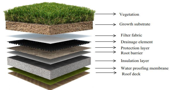
Fig. 1 Components of a green roof [8].
