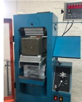
Fig. 3 Universal Machine, running bending test on specimen M2
