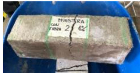
Fig. 9 M2 test tube with 1% fiber incorporation
