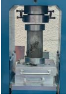
Fig. 10 M3 specimen without fiber incorporation
