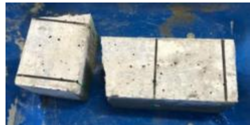
Fig. 8 M1 test tubes without fiber dosage
