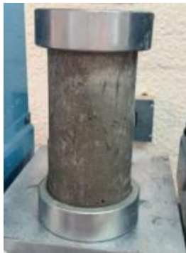
Fig. 11 M4 test tube with 1% fiber incorporation
